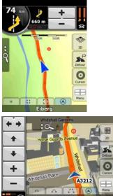
During navigation, the screen shows route information and trip data (left screenshot), but when you tap the map, additional buttons and controls appear for a few seconds (right screenshot). Most parts of the screen behave as buttons.
