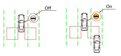
C. Turn on right indicate light, there is a car in the detection area, warning LED will keep flash and buzzer will give out "bi-bi" warning;
