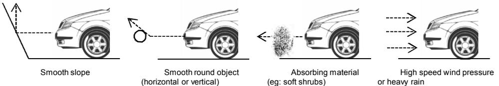
At the time of installation, an on/off switch may have been fitted within easy reach for the driver. In situations where wind pressure is an issue, or the sensors detect other vehicles in traffic jams, or any of the above situations, the sensors can be turned off to prevent any annoyance. Please remember to turn them on when parking.
