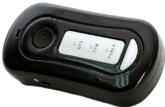
The PT301 is a personal/portable GPS tracker using satellites to calculate its precise location and both GSM and GPRS technology for communications. The tracker is also a non-dialing emergency 2 way mobile phone which can be used to summon help or assistance.
